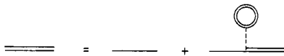
Figure 1. Graphical equation for the Hartree propagator g(k) . A single full line represents the bare propagator g_0(k) .
